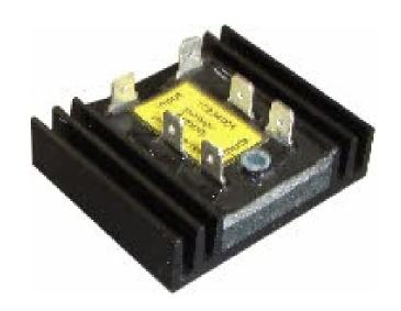
Diode pack provides the radar and other sensitive equipment a clean power supply when the engine is being started from the common service / start battery bank.
