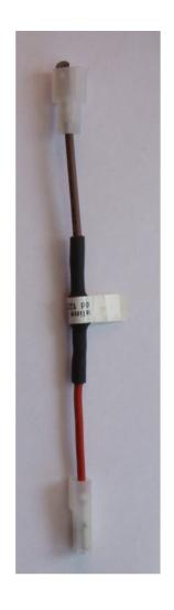
Diode assembly, plugs into bilge pump feed from manual switch, prevents back feed from auto operation. Sealed with adhesive lined shrink tube for mechanical strength and protection water and atmosphere.
