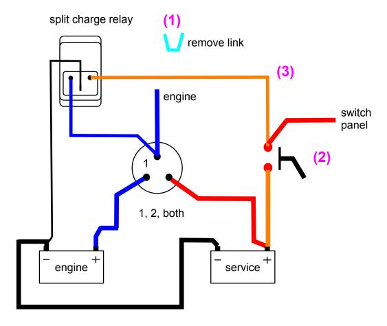
To correct the installation fit a new isolator (2) and fit a new link cable between isolator and service battery positive, using suitable size cable. Transfer feed to service loads from the 1,2,both switch to the new isolator.
