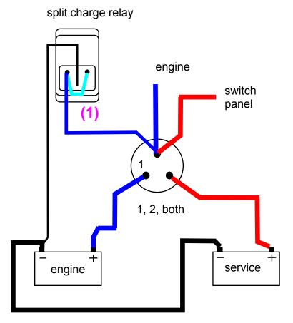
When built the boat should been been fitted with two isolator switches, one for engine supply, one for service power supply. A feed from each switch should have gone to the split charge relay, supplying feed to each voltage display and providing split charge.
