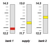
display ... voltage for two battery banks off load, provides battery capacity indication and reserve in bank that is not in use, plus recharge voltage.
